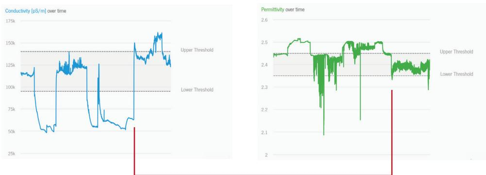
You can keep a close-up follow of live information on contamination, and / or chemical changes inside the oil due to other incoming impurities such as water, wrong oil type, additive reactions, etc.
